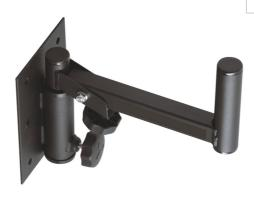
Heavy duty wall mount bracket for loads up to 40kg. It is slewable for 180° and tiltable from 90° to 110° downwards, The complete system is from black powder coated 2mm steel, length: 29cm, base plate: 20 x 15 cm, weight: 2,10kg
