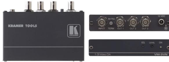
The VM-3VN is a distribution amplifier for composite video signals. The unit takes one input, provides correct buffering and isolation and distributes the signal to three identical outputs.
