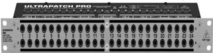
Professional patchbay eliminates cable clutter in your studio and adding order and clarity. Fully balanced high-quality?" TRS connectors. 3 modes, easily selectable per channel via top-side switches. interconnects the two rear jacks of one channel; inserting a plug into one of the front jacks interrupts the connection of the rear jacks.
