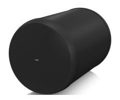
Pendant loudspeaker Coaxial 2 way, with woofer 8" and ferrofluid cooled neodymium tweeter 0.75 ". 60-30-15-7,5 watt @ 100 & 70 V or 70W @ 16 $\Omega$ . Conical dispersion 80°. Frequency response 60-30000Hz, sensitivity 90dB / W / m, 114dB max Weight 7,8 kg, Black color. Safety removable connector, with screw terminals and loop through facility. For indoor & outdoor use, weather resistant to IP64.
