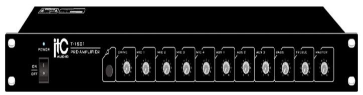
The T-1S01 is a public address pre-amplifier with five balanced MIC inputs, three AUX level inputs and one EMC (priority) level inputs. Priority muting is achieved via MIC 1 and EMC 1 for overriding music for paging and emergency alarms. Individual gain controls are provided for MIC and AUX inputs, bass and treble controls are provided for overall tone control.
