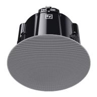
8'' ceiling subwoofer  $70/100\text{V}-8\Omega.$  Frequency range 45-380Hz, omnidirectional coverage (360°), continuous power 180W, peak 720W. Dimensions Ø 353mm × depth 350mm, mounting depth 240mm, weight 7.25kg, in white color. Black coloured replacement grill available.
