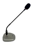
Condenser Microphone , Phantom power 48V & DC3V , balanced output , ABS base , XLR output
