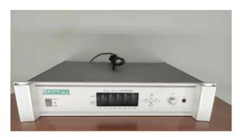
Audio matrix 8x8. Inputs: 1 x EMC, 8 input channels & amp; amp; 8 output channels.
