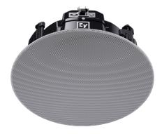
6,5" two-way coaxial ceiling speaker for 70/100 V or 8  $\Omega$  use, designed for low ceilings. Frequency response down to 60 Hz, peak SPL 115 dB. Diameter 353 mm, weight 4.5 kg, in white color. Black coloured replacement grill available.
