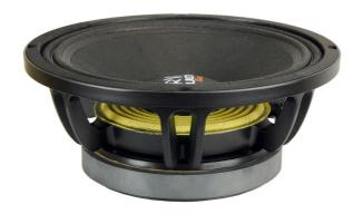
The PRV Audio 10MB800 mid-bass woofer offers outstanding durability and high power handling. This is one of the best selling pro audio speakers from the PRV line. A specially designed dual spider suspension is assembled with a special resin improving the resistance against failure during intense use. The M-Roll surround offers smooth accurate geometry during hard play.
