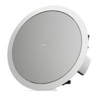
In-ceiling subwoofer100W @  $6\Omega$  or 60-30-15-7,5 watt @ 100 & 70 V. Frequency response 42-300Hz, sensitivity 92dB / W / m, 118dB max. The woofer is without enclosure. Option BACKCAN CMS801 PI. Cutout diameter 295mm. Baffle diameter 325mm and depth 123,7mm. Weight 3,2 kg. Safety removable connector, with screw terminals and loop through facility
