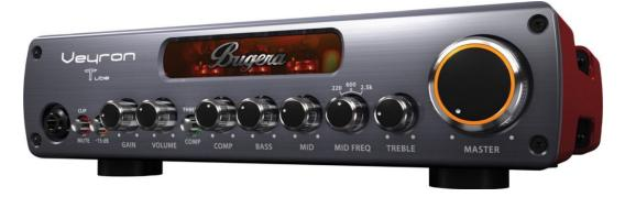
Ultra-high power, ultra-lightweight 2,000-Watt bass amplifier driven by 3 x 12AX7 vacuum tubes. 6-stage Class-A tube preamplifier. Dedicated Bass, Mid and Treble controls. Selectable mid-frequency switch provides 3 classic sound variations. Balanced DI output with pre/post EQ. Passive Baxandall bass and high band EQ plus active tube-driven mid EQ.
