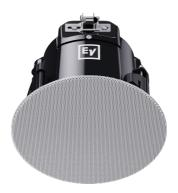
4" two-way coaxial ceiling speaker for 70/100 V or 8  $\Omega$  use. Frequency response down to 70 Hz, peak SPL 112 dB. Measures Ø 201 × 176 mm deep, weighs 2.7 kg, in white color. Black coloured replacement grill available.
