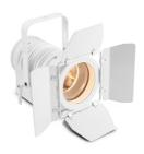
. A powerful 40W warm white LED spotlight with a plano-convex lens and manual zoom, offering a 14°-38° beam angle. Delivers 18,000 lux at 1m with a 3,200K color temperature and CRI >90 for excellent color rendering. RDM-capable with flicker-free operation. Features rugged metal housing with convection cooling and includes rotatable barn doors and a filter frame
