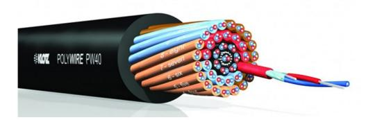
Analog audio multicore 12 pair PolyWIRE cable with 0.22mm² cross section. Designed for studio & performance with compact dimensions. The high conductor cross-section of 0.22mm² prevents signal attenuation and can easily handle transmission over long distances. Overall diameter 15 mm. Weight 260 grm/mtr. Black color.
