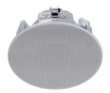
3" coaxial ceiling speaker with frequency response 90Hz-19kHz, 40W continuous power & 160W peak, max. SPL 106dB peak / 100dB continuous, 70/100V lines (0.9/1.88/3.75/7.5/15W) & 8 $\Omega$ . Coverage angle 135°, Mounting cut-out Ø 183mm, depth 98.3mm, weight 2.1 kg, IP45 rated, in white color. Black coloured replacement grill available.
