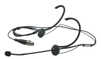
Headworn supercardioid microphone ideal for vocal. Audio Frequency Response 50 - 20,000 Hz, Maximum SPL (1% THD) 115 dB.
