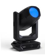
IP65 Spot Profile Moving Head with 300W LED and 11,000 lm output. Features motorized framing blades (±60° swiveling), 3°-50° zoom, CMY color mixing, and an 8-filter color wheel. Includes a rotating gobo wheel with 7 replaceable glass gobos, overlapping circular prisms, and linear CTO for precise color tuning. Offers selectable PWM up to 25 kHz for flicker-free operation and quiet performance with three noise modes.
