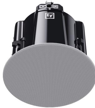
8-inch full-range coaxial speaker, 70/100V or 8Ω. Frequency range 50-20k Hz, max SPL 119dB. Diameter 300 mm, depth 255mm, weight 5kg, in white color. Black coloured replacement grill available.
