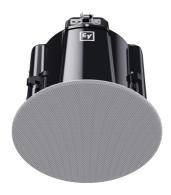
8-inch full-range coaxial speaker, 70/100V or  $8\Omega$ . Frequency range 50-20k Hz, max SPL 119dB. Diameter 300 mm, depth 255mm, weight 5kg, in white color. Black coloured replacement grill available.
