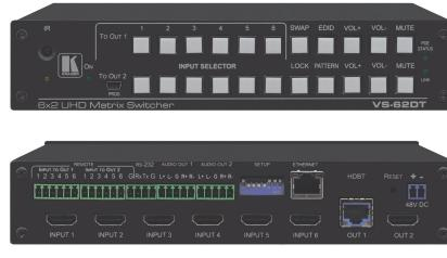
VS-62DT is a 6x2 4K@60Hz (4:2:0) HDMI/HDBaseT matrix switcher with HDMI and HDBaseT output transmitters that provide long-reach video and audio transmission. It supports resolutions of up to 4K@60Hz (4:2:0) and WUXGA. The matrix is a PoE provider that provides power over Ethernet to compatible PoE receivers.
