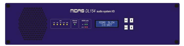
The DL154 delivers legendary MIDAS sound quality in a cost effective, discrete 2U chassis that utilises time-tested and proven MIDAS technologies. Equipped with 8 channels of MIDAS premium mic-pre amplifiers with 2.5 dB gain steps and 16 balanced line level outputs, selectable sample rate and dual redundant AES50 network ports the DL154 is the ideal partner to the PRO 1 and PRO 2 digital consoles — significantly increasing the network capacity and number of mic. inputs and analogue outputs.
