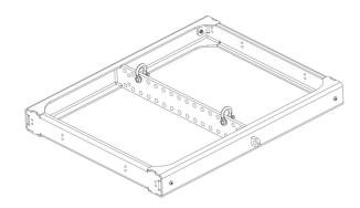
Flying frame for vertical deployment of A15i and KS21i.
