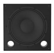
In-ceiling subwoofer 12" 200W @  $8\Omega$  or 150-75-38-19 watt @ 100 & 70 V with option transformer. Frequency response 30-3000Hz, sensitivity 93dB / W / m, 126dB max. The woofer is fits on a baffle made by 1.2 mm black powder coated steel. Weight 9.0 kg. Dimensions (W x D) 588 x 457mm. Safety removable connector, with screw terminals and loop through facility
