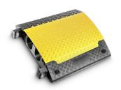
Heavy-duty cable crossover made of black, recyclable polyurethane for demanding applications. 6 channels: 2 channels 108 x 110 mm, 4 channels 25 mm in diameter. Load bearing capacity approx. 5 t / 20 x 20 cm. Dimensions 70 x 76.6 x 12 cm. Weight 28.295 kg.
