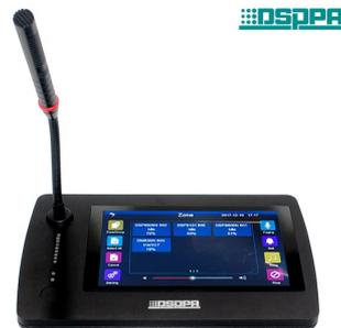
7" TFT true-color LCD touch screen. Up to 200 partitions. Five-point touch control. Energy-saving operation. Remote upgrading pushed by the host. 1 Aux input& output, 2 MIC input, 1 EMC output, and 1 short circuit output
