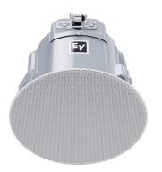
4" coaxial ceiling speaker. Frequency range 80Hz-20kHz. Continuous power 50W, peak 200W. Max. SPL 112dB, continuous 106dB, 1.25/2.5/5/10/20W & 8 $\Omega$ . Coverage angle 130°, mounting cut-out Ø 183mm, depth 163.4mm, weight 2.6 kg. For indoor use, safety certifications and UL ratings included, in white color. Black coloured replacement grill available.
