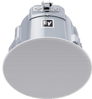
4" coaxial ceiling speaker. Frequency range 80Hz-20kHz. Continuous power 50W, peak 200W. Max. SPL 112dB, continuous 106dB, 1.25/2.5/5/10/20W & 8Ω. Coverage angle 130°, mounting cut-out Ø 183mm, depth 163.4mm, weight 2.6 kg. For indoor use, safety certifications and UL ratings included, in white color. Black coloured replacement grill available.
