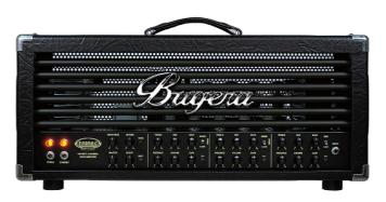
Hand-built and hand-wired 100-Watt Class A/B amplifier driven by 4 x 6L6 tubes. 3 fully independent channels with switchable killer voicings (Classic, Vintage and Modern) featuring 5 x 12AX7 tubes. 3 unique rectifier modes featuring 2 x 5U4 tubes and silicon diodes for ultimate performance. Integrated high-class reverb with dedicated Reverb control. Dedicated Gain, Bass, Mid, Treble, Presence and Volume controls per channel. Adjustable and remote controllable Boost function for ultimate punch.
