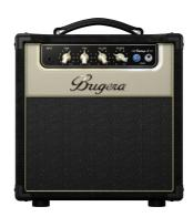
Hand-built 5-Watt Class-A amplifier driven by 1 x EL84 tube Way cool vintage look and feel Original 8" BUGERA guitar speaker for true vintage sound Authentic preamp design from the 60s featuring 1 x 12AX7 tube—everything from purring blues to mind-blowing crunch Integrated high-class reverb with dedicated Reverb control Vintage Equalizer with dedicated Tone control Built-in 2-way Power Attenuator allows you to get ultimate sound at any volume
