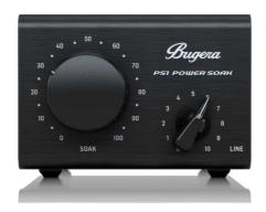
Passive 100-Watt Power Attenuator allows you to get the ultimate overdriven tone at any volume. Multi-impedance input connectors (4, 8 and 16 Ohms) to match virtually any amplifier. Line output with dedicated Level control. Emulated Mic Output mimics a microphone in front of a speaker cabinet.
