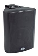
5"+1.5" Two way wall mount speaker, 3.75W-7.5W-15W-30W@100V+80hm, ABS body, metal grille, metal bracket, black.
