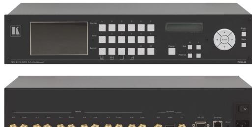
The MV-6 is a versatile, high-performance multiviewer for 3G HD-SDI video signals. The device can display up to six inputs in any combination and output the image in SDI, HDMI and CV formats. Both pre-programmed and customizable screen divisions are supported. The MV-6-MD is certified for medical applications.
