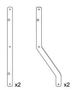
End rear rigging plates for A15i and A10i onto or under KS21i.
