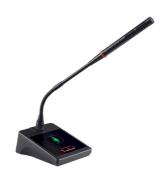
XLR jack,Plug & play, easy to use Sensitivity: -40dB±2dB Wide frequency response: 40Hz-16kHz •Output impedance: 200Ω •Directivity Ultra-cardioid •Pice up distance:10-50cm •Condenser Microphone •Power supply:DC4.5V/Phantom 48V •Working time: 24h (AA battery x2pcs)
