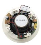
The Galil 6–CO is a pair of two-way open-back  $8\Omega$  speakers designed for mounting in the ceiling. The speakers feature a multi-tap power transformer for selecting direct  $8\Omega$  (bypassing the transformer) or 70V/100V power settings suitable for array installation.
