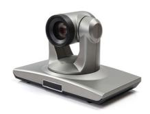
HD Video-Conferencing Camera. Image Inductor 1/3" High quality HD CMOS inductor, Effective Pixels - Motion picture:16:9,2.07megapixel Static picture:16?9, 2.1megapixel, Video Signal 1080P60/50/30/25, 1080I60/50, 720P60/50/30/25. Zoom rate: 18 x optical, f=f=4.7~84.6mm, Angel of view: wide:55°,tele:3.8°, Sensitivity: 1.8Lux, White balance: Auto/Manual, Focus: Auto/Manual, Iris: Auto/Manual, Gain control: Auto/Manual, Balance Compensation: Auto/Manual, Signal-to Noise: & amp;gt;50dB
