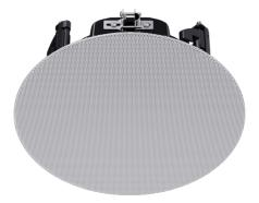
4" two-way coaxial ceiling speaker for 70/100 V or 8  $\Omega$  use, designed for low ceilings. Frequency response down to 80 Hz, peak SPL 112 dB. Measures Ø 269 × 94 mm deep, weighs 3.32 kg, in white color. Black coloured replacement grill available.
