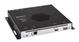
AV over IP decoder that transports 4K60 4:4:4 video over standard Gigabit Ethernet A reliable, high performance AV over IP decoder that receives 4K60 4:4:4 video over standard Gigabit Ethernet with no perceptible latency or loss of quality. Supports HDR10 and HDCP 2.2. Provides a secure 4K signal routing solution for enterprise and campus wide content distribution applications.
