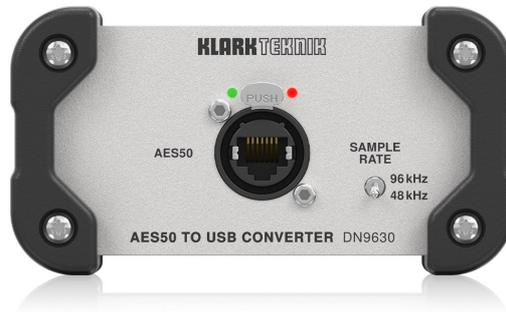
AES50 to USB 2.0 converter for simultaneous computer audio recording and playback. Up to 48 bidirectional channels @ 48 kHz and 24 bidirectional channels @ 96 kHz. Switchable 48 kHz and 96 kHz sample rate operation. Operates from incoming AES50 clock. Powered via USB 2.0 interface. Native Core Audio\* driver support in Mac OS X\*, software drivers available for Windows\* PC. LED indicators monitor network activity and speed.
