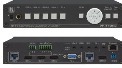
VP-440H2 is a high-performance 4K@60Hz (4:4:4) presentation scaler/switcher with one HDBaseT/POE, three HDMI and one computer graphics (VGA) inputs. The unit scales the video, embeds the audio and outputs the signal to an HDMI and an HDBaseT output simultaneously. The unit includes analog and embedded audio inputs and outputs.
