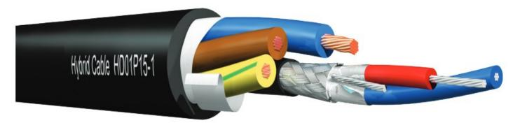
Hybrid cable to cabling active speakers, dimmers, colour changers and scanners. 1 signal cable (DMX, digital audio, analog audio), 1 power cable (3 X 1,5). Overall diameter 15,4 mm. Weight 220 grm/mtr. Black color.
