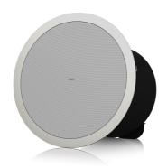
Two Way In-ceiling full bandwidth Coaxial Loudspeaker, 60-30-15-7,5 watt @ 100 & 70 V or 60W @ 6 $\Omega$  with woofer 8" and ferrofluid cooled neodymium tweeter 0.75 " Conical dispersion 90°. Frequency response 60-24000Hz, sensitivity 93dB / W / m, 117dB max Weight 6.5 kg, white color, Hole Cutout Diameter 250mm Safety removable connector, with screw terminals and loop through facility
