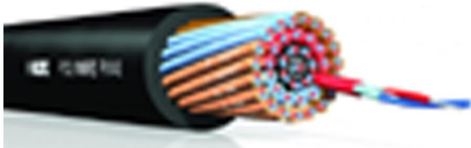
Analog audio multicore 2 pair PolyWIRE cable with 0.22mm<sup>2</sup> cross section. Designed for studio & installation use, successfully combines superb performance with compact dimensions. The high conductor cross-section of 0.22mm<sup>2</sup> prevents signal attenuation and can easily handle transmission over long distances. Overall diameter 8 mm. Weight 65 grm/mtr. Black color.
