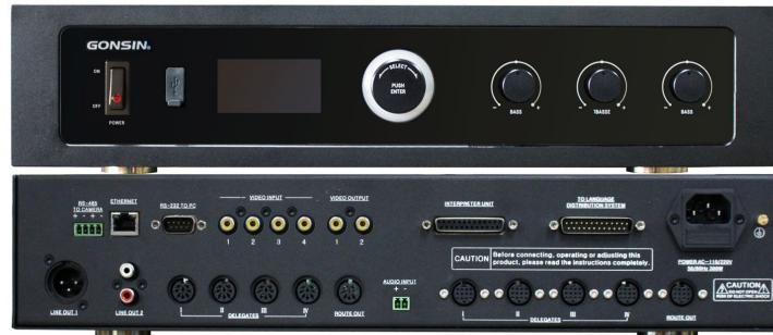
Central Control Unit . Main features in stand-alone mode: 1 to 4 delegate microphones can be active simultaneously, Selectable microphone mode: AUTO/FIFO/OPERATOR, ID number writing for each unit using LCD on front panel, Automatic video tracking with up to 4 dome cameras, Built-in DSP processor for acoustic feedback prevention, Built-in treble/bass compensation for better sound quality, Built-in MIC IN audio input for wireless mic system
