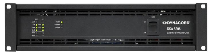
The next generation of Contractor Precision Series two-channel amplifiers provide flexibility and reliability for the professional installation business. Designed for the contractor, the DSA8206 feature 2-RU chassis, Phoenix-type connectors for inputs and outputs, preprogrammable power-on delay, easy power-on via remote contact closures, rear panel attenuators, and a switchable 50 Hz high-pass filter (HPF).
