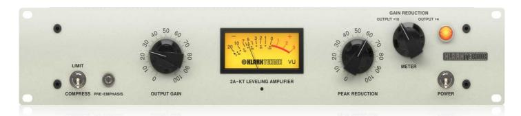
Classic Leveling Amplifier with Vacuum Tubes, Optical Attenuator and Midas Transformers. Completely discrete signal path. Premium selection 12AX7, 12BH7 and EL84 tubes. Lag-free optical attenuator based on original electroluminescent technology. Gain Limiting: 0 to 30 dB. Ultra-fast attack time: 10 milliseconds. Release time: 50 milliseconds to 5 seconds. Adjustable stereo-link connection. Designed and engineered in the U.K.
