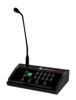
Remote Zone Paging Console works with T-6212(A), max 160 zone, CAT 5 cable system.
