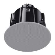
8'' coaxial speaker designed for high ceiling environments, 70/100V-  $8\Omega.$  Response 60 Hz-20k Hz, max SPL 124 dB. Dimensions Ø 353mm × depth 350mm, mounting depth 240 mm, weight 6 kg, in white color. Black coloured replacement grill available.
