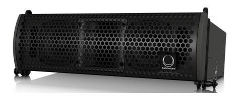
Compact Biamp 2 Way Line Array loudspeaker, with 2x4" Kevlar woofer 150W @  $16\Omega$  and 1x1,0" HF driver 30W @  $16\Omega$ . Dispersion 120° x 10°. Frequency response 70-20000Hz, sensitivity 87dB / W / m, 109dB max. Black color. Dimensions (HxWxD) 163 x 512 x 290 mm. Weight 8,0 kg
