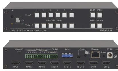
The VS-62H is a high-quality, 6x2 matrix switcher for 4K UHD HDMI signals. It reclocks and equalizes the signals and can route any input to either or both outputs simultaneously. It supports resolutions up to 4K@60Hz (4:2:0) UHD and WUXGA.
