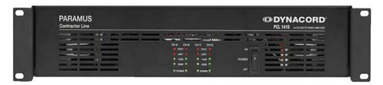
The PCL1415 is from the PA series of professional commercial audio amplifiers. The direct-path airflow design significantly reduces heat buildup, and allows four full amplifier channels in a slim, two-rack space chassis. The superior audio performance of the PCL1415 fulfills the requirements of many demanding, long-term applications such as sound reinforcement, paging, or life safety installations
